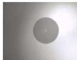
Image viewed through coaxial illumination below shows clean connector downloaded from SD card with time and date of image capture
